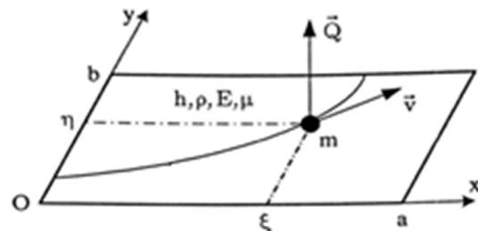
Figure 1. Plate element under moving load.
