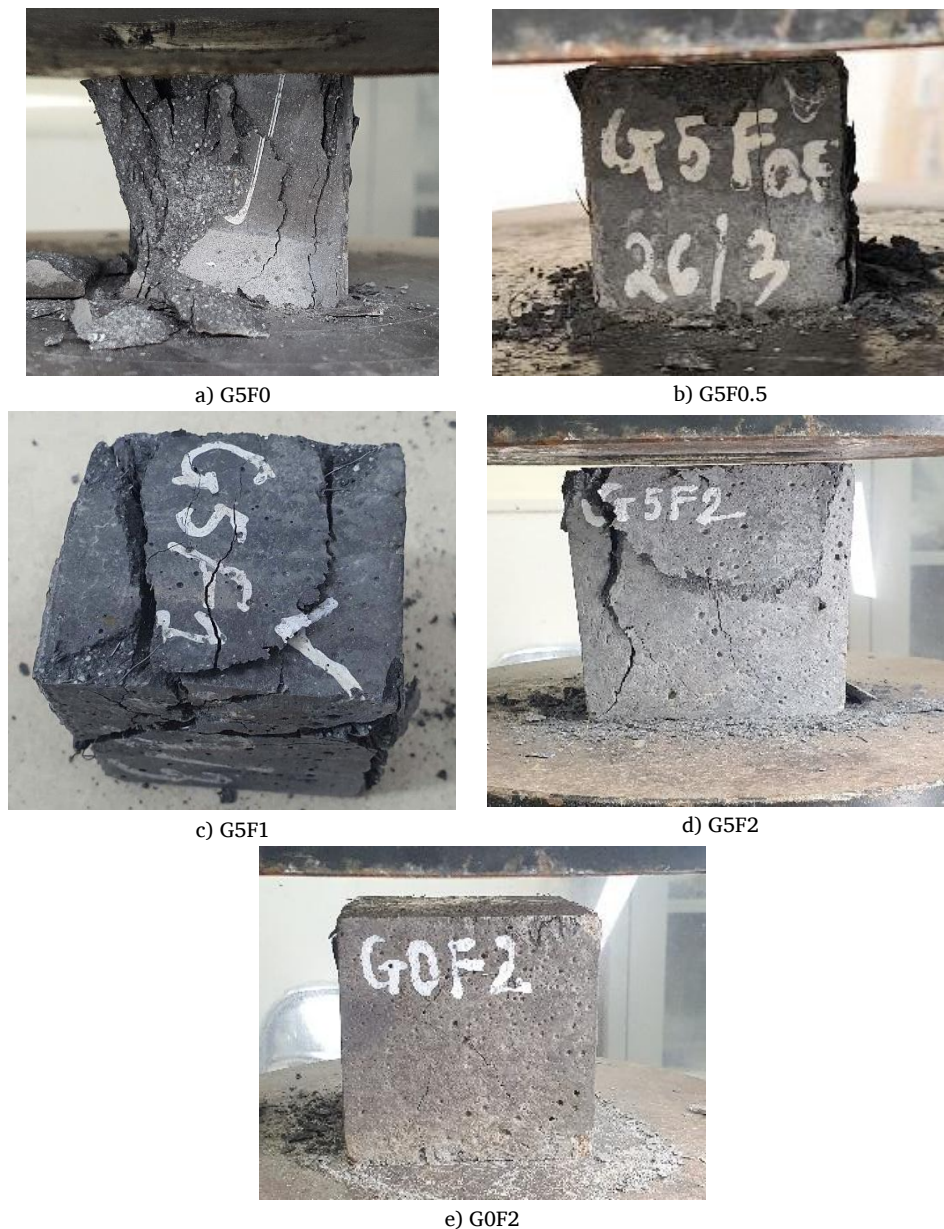
Figure 3. Fracture images of SHPCs under compression.
