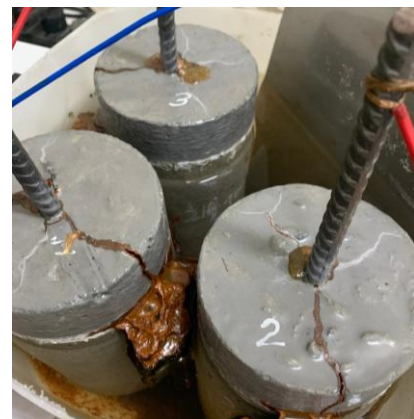
Figure 7. Steel corrosion causes concrete cracking.
