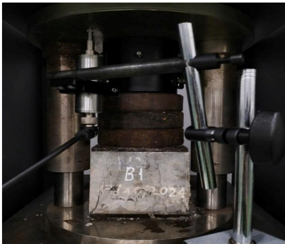
c) Crack formation during the loading process
