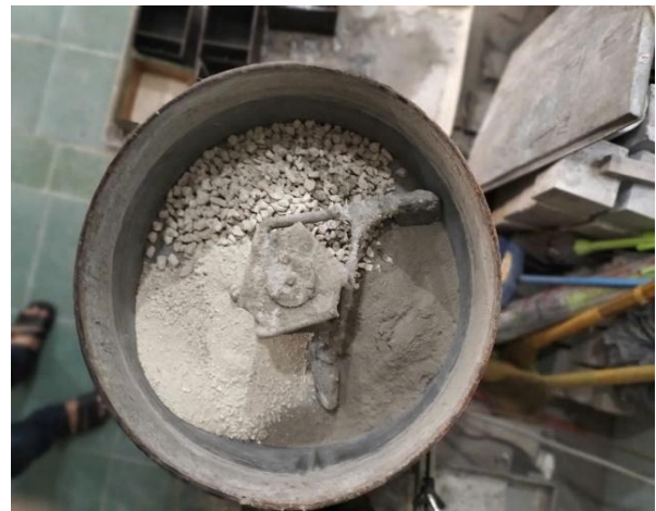
b) Mixing of coral concrete
