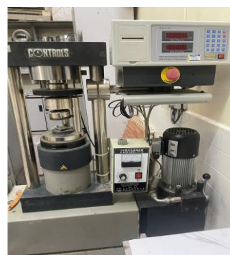
Figure 11. The compressive strength testing machine manufactured by Controls.
