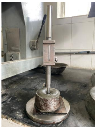
Figure 7. Vicat apparatus is used to determine the standard water content of cement samples.
