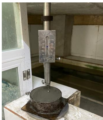
Figure 9. Vicat apparatus is used to determine the final setting time.
