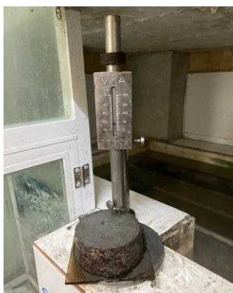
Figure 8. Vicat apparatus is used to determine the initial setting time.
