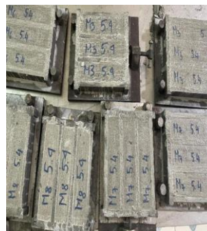
Figure 10. Mortar samples in mold with dimensions of 40 mm × 40 mm × 160 mm.
