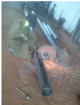
a. Steel tube cutting
