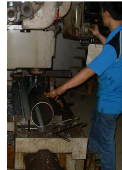
c. Hole drilling
