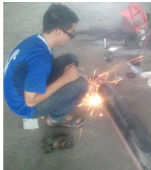
b. Surface grinding
