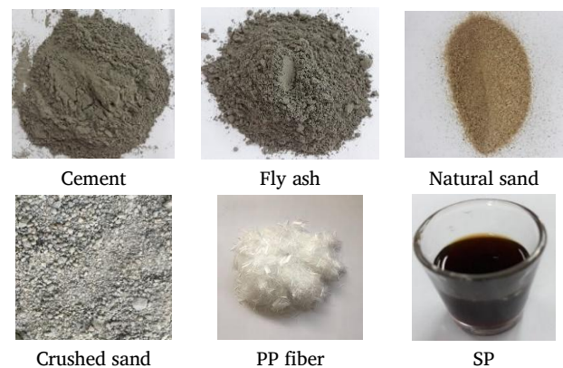
Figure 1. Ingredients of fiber concrete.
