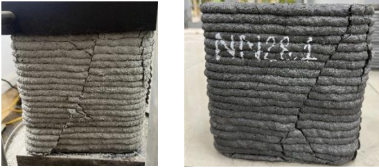
Figure 8. Inclined cracking failure in 3D-printed concrete.
