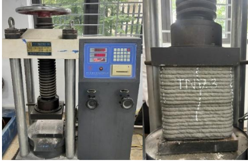
Figure 5. Compression test of 3D-printed concrete samples.
