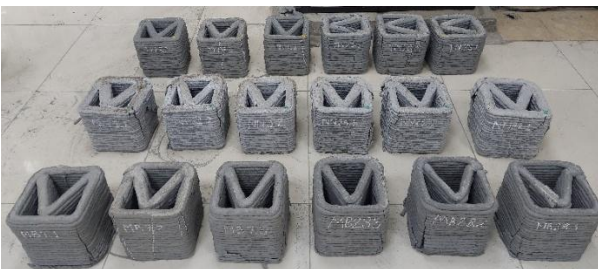
Figure 9. Cracking patterns of 3D-printed concrete samples.
