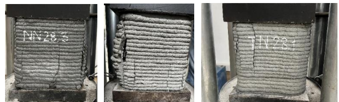
Figure 7. Vertical cracking failure in 3D-printed concrete.
