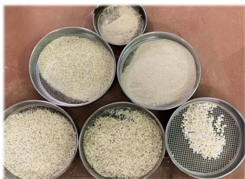
Figure 4. Oyster shells are crushed and sieved with a grain size range of 0.14 – 5 mm.
