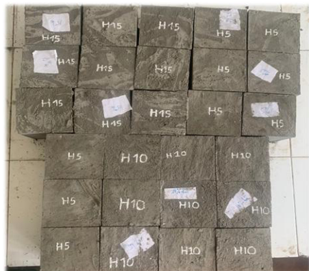
Figure 7. The curing of concrete samples.
