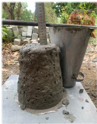
Figure 6. Measuring the slump of concrete mixtures.
