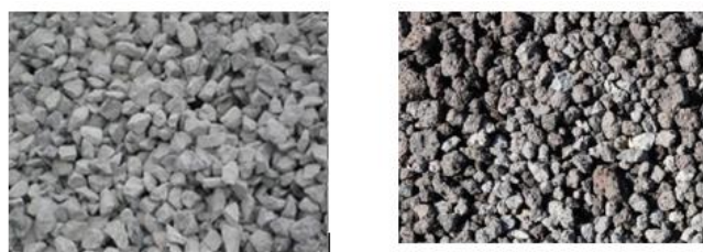
Figure 2. Crushed Stone (left) Compared with Steel Slag (right).
