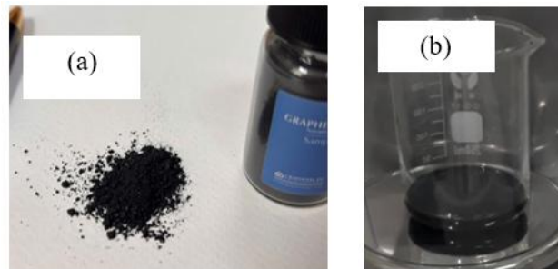
Figure 1. Graphene-based nanosheets under powder (a) and liquid (b) forms.
