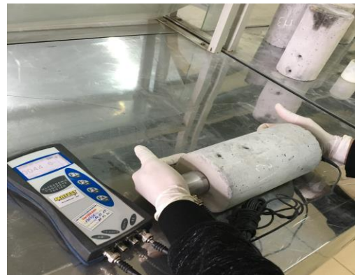
Figure 4. Testing of measuring ultrasonic pulse velocity in concrete.
