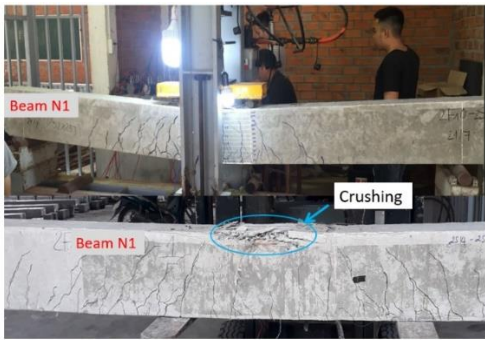
Figure 18. Cracking and crushing in the test.
