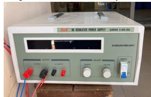
Figure 10. DC power for corrosion test.
