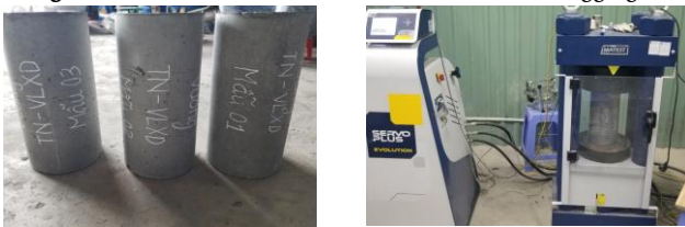
(a) cylinder specimens (b) Testing compressive strength
