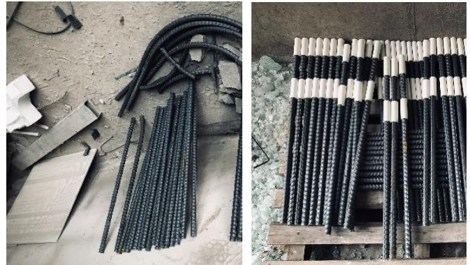
(a) Cutting steel bars (b) Determining corroded segment
