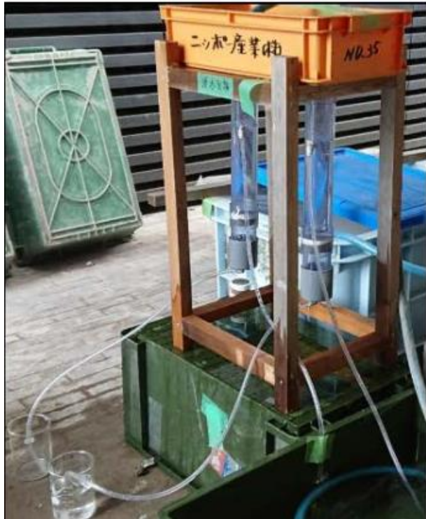
Figure 7. The first generation of water flow testing system developed in this study with multi-function for multi-parameter studying.
