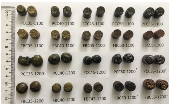
Figure 6. Bloating of aggregates fired at 1000 °C and 1200 °C.
