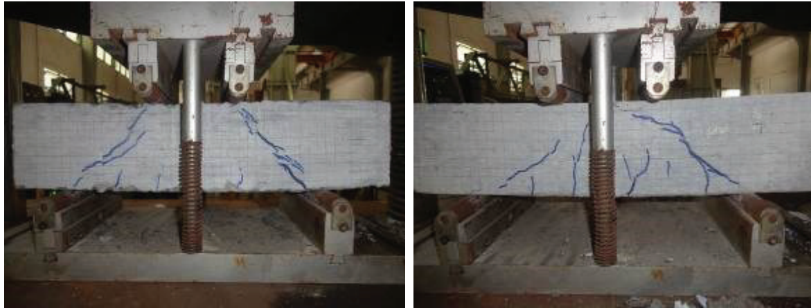
Figure 7. Bending test of specimen M250, M400 at peak load.
