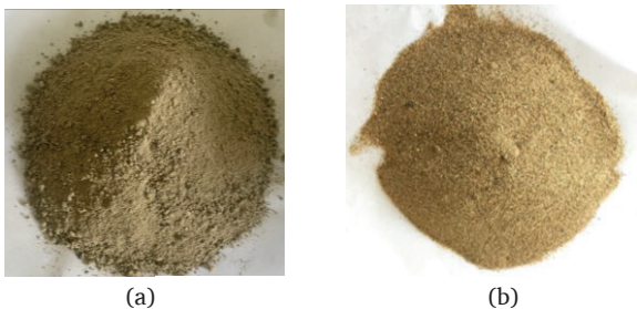
Fig. 1. The appearance of materials: (a) bottom ash; (b) river sand.
