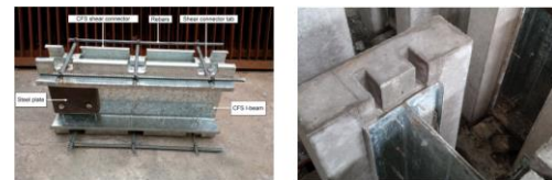
Figure 1. Specimen before and after concreting.
