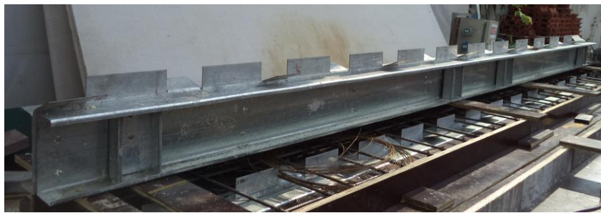
Figure 1. Practical image of cold-formed steel and perfobond shear connectors.
