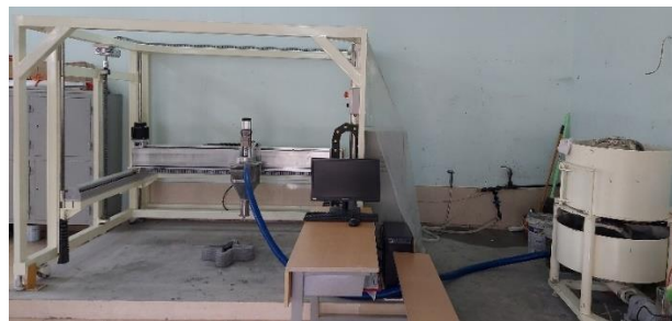
(b) Overview of concrete printer and mixing/pump system
