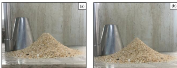
Figure 3. The shape of the aggregate under the (a) OD and (b) SSD states.
