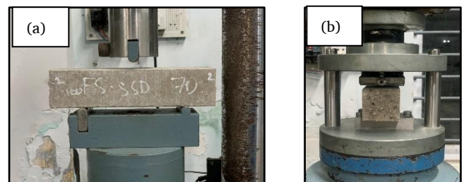
Figure 5. Testing (a) flexural and (b) compressive strength of cement mortar.
