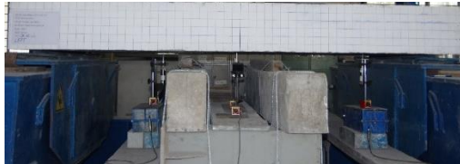
b. Installation of LVDT1, LVDT2, LVDT3
