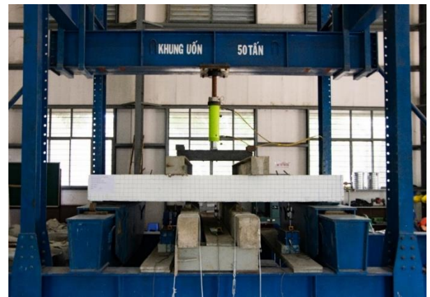
Figure 10. Arrangement of the test slab specimens.
