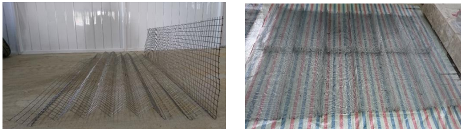
Figure 6. Steel grating after bending forming.
