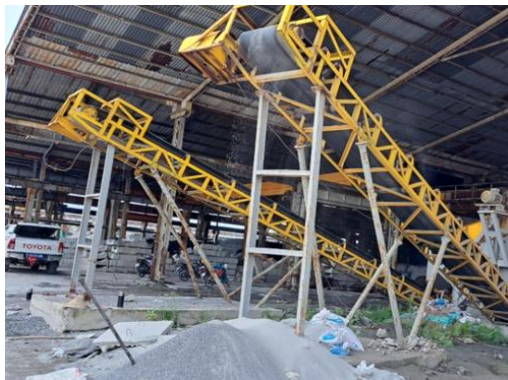
(a) Crushing process of concrete waste to produce sand
