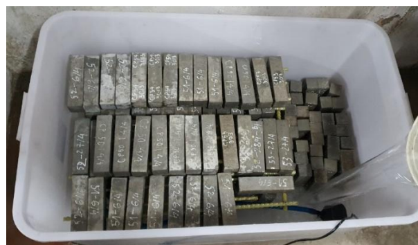
Figure 2. Curing mortar samples in wastewater environment.
