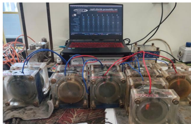
Figure 8. Chloride ion penetration test.
