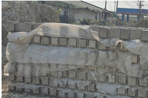
b. Salt-resistant concrete piles
