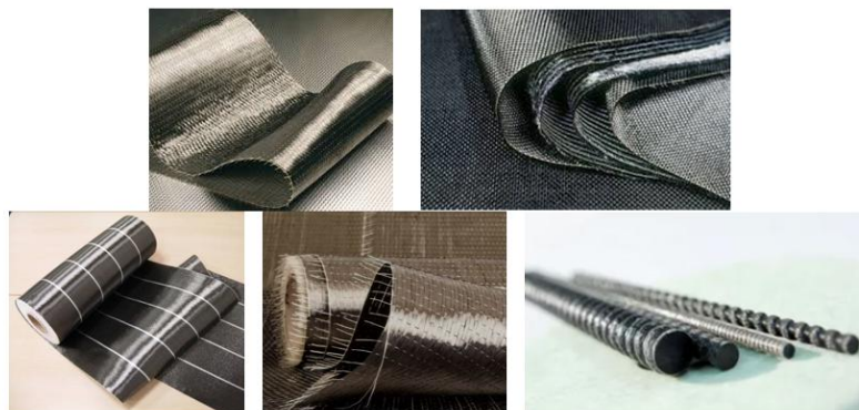
Figure 1. FRP fiber material reinforcing reinforced concrete structures [1].
