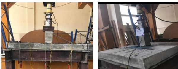
Fig.1. Column placed directly on slab reinforced with GFRP [6].
