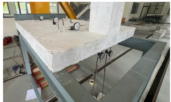
Figure 3. Slab positioned on the test platform with the column at the free edge.
