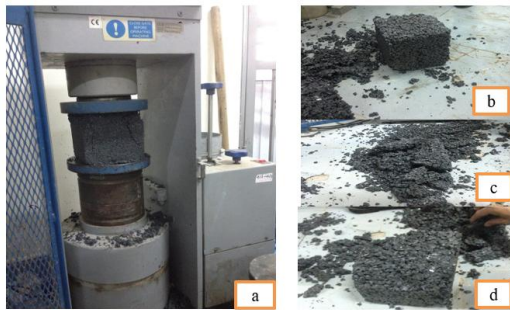
Fig 11. a- Compressive strength test; b,c,d - damaged samples after test.
