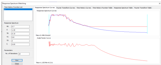
Figure 8. Time scaling chart based on the elastic response spectrum in TCVN 9386:2012.
